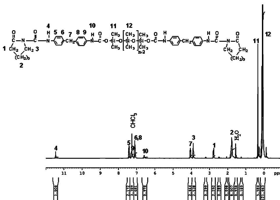
Figure 5 ^1\text{H-NMR} analysis of \alpha,\omega -dicarbamoyloxy caprolactam PDMS (Macroinitiator 1).
